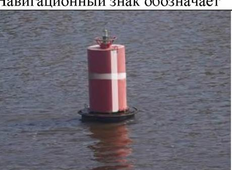
A red cylindrical buoy with a single white horizontal band, mounted on a black circular float.                                            |
