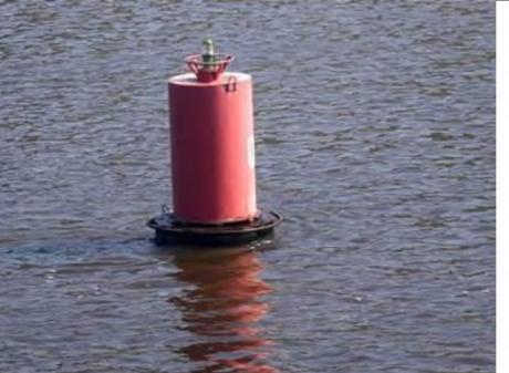
A solid red cylindrical buoy floating in water, mounted on a black circular float.                                                         |
